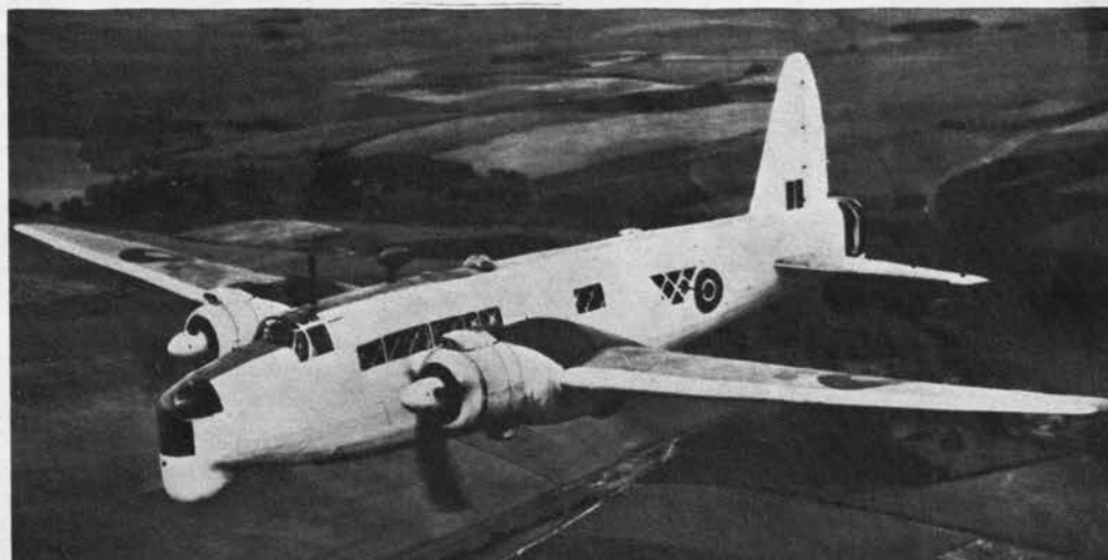
Wellington XIV has no nose turret but carries a radar installation under the chin. A retractable Leigh Light, which is used on search and patrol missions, is carried in the bomb bay.
